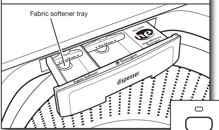
Pour a measured amount of liquid fabric softener into tray, always follow manufacturer's directions for correct amount of fabric softener based on your load size. Close dispenser drawer, then select Fabric Softener option.
