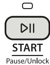
Press the START/Pause/Unlock button to start the wash cycle. When the cycle has finished, the DONE indicator will light. Promptly remove garments after cycle has completed to avoid odor, reduce wrinkling, and rusting of metal hooks, zippers, and snaps.
