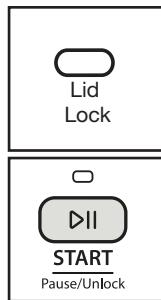
If you need to open the lid, press START/PAUSE/UNLOCK. The lid will unlock once the washer movement has stopped. This may take several minutes if the load was spinning at high speed. Press START/Pause/Unlock again to resume the cycle.
