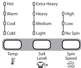
Once you select a cycle, the default settings for that cycle will be lit. Press the cycle settings buttons to change the Temp, Soil Level, and Spin Speed, if desired.
